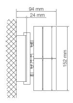
Lamp type: high-voltage halogen lamp Recommended lamp: Osram Halopin 25 W, 230 V
