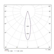
Lamp type: low-voltage halogen lamp Lamp denomination: Osram Decostar 51 IRC pin base GU5.3 Base: Diameter: mm 12 V Voltage: Power: 35 W Depth of insertion: 100 mm 1 - 15 mm Ceiling thickness: Ø 65 mm Ceiling opening: Product weight: 300 g
