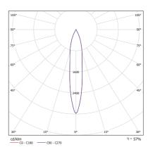
Lamp type: low-voltage halogen lamp Lamp denomination: Osram Halostar IRC 50 W
