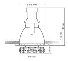
Lamp type: high-voltage halogen lamp Osram Halolux Ceram 100 W Lamp denomination:
